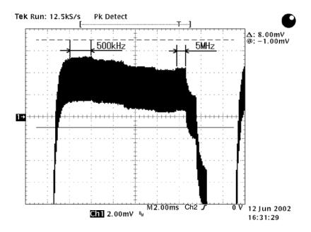
Figure 3-4: Verifying the signal amplitudes from 500 kHz to 5 MHz
